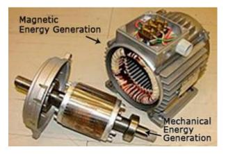
transformation of the magnetic force into mechanical energy. These processes happen within the rotor and the stator of an electric motor.
